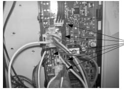
Step 3. Unplug wire connections from board and replace.
